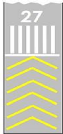
Pre threshold area fit for use by aircraft as a stopway only
